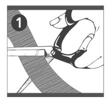
1. Cut the edgebanding 3 cm longer than surface to be covered. Make sure the surface is dust-free, clean, and dry. Also check to see there are no rough spots on the surface.
