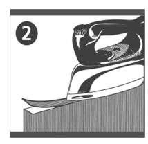
2. Apply the edgebanding with hot iron or hot air blower as described. It is recommended to use paper to protect iron bottom
