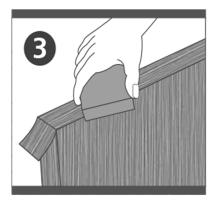
3. While still hot, press firmly with a wood block to the board.
