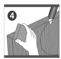
4. Allow the edgebanding to cool completely, remove the extra edges with a trimmer or a cutting blade and sand the edges.
