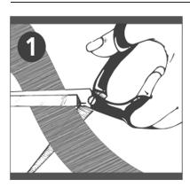
1. Cut the edgebanding 3 cm longer than surface to be covered. Make sure the surface is dust-free, clean, and dry. Also check to see there are no rough spots on the surface.
